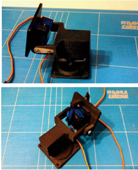
Figure 8. View of the tracking system that makes use of servo motors to follow the Sun.
