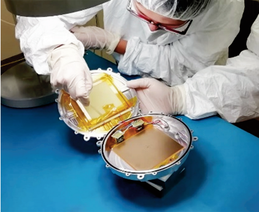
Figure 5. Integration of the Micromegas at the INFN (National Institute of Nuclear Physics) laboratory in Pisa.
