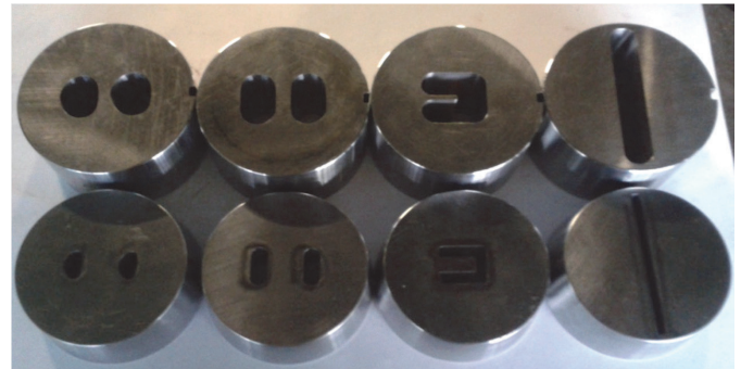
Fig. 6. The dies and backers (above) for extrusion of solid sections
