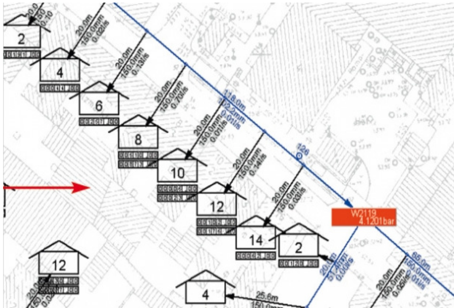
Fig. 1. Diagram of a water supply network in the STANET application [3]
