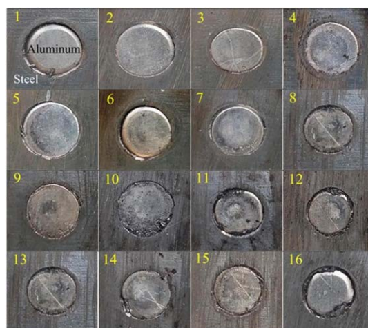
Fig.4. Extruded aluminum through steel hole.
