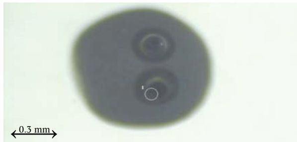
Fig. 2. Photo of a microsphere with spherical zirconia particle \Phi = 1 mm after laser evaporation.
