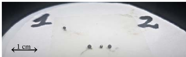
Fig. 1. LA stand with SiC (outer) and Zr (middle) spheres. Numbers allow positioning of the table in relation to the beam.
