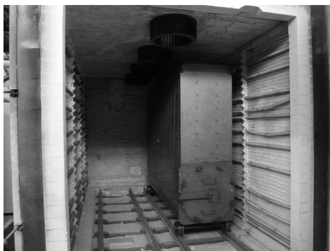
Fig. 2. Pyrolysis plant PTR 1000 (HEDVIGA GROUP plc) – thermal module with so called fuel cell [8, 9]
