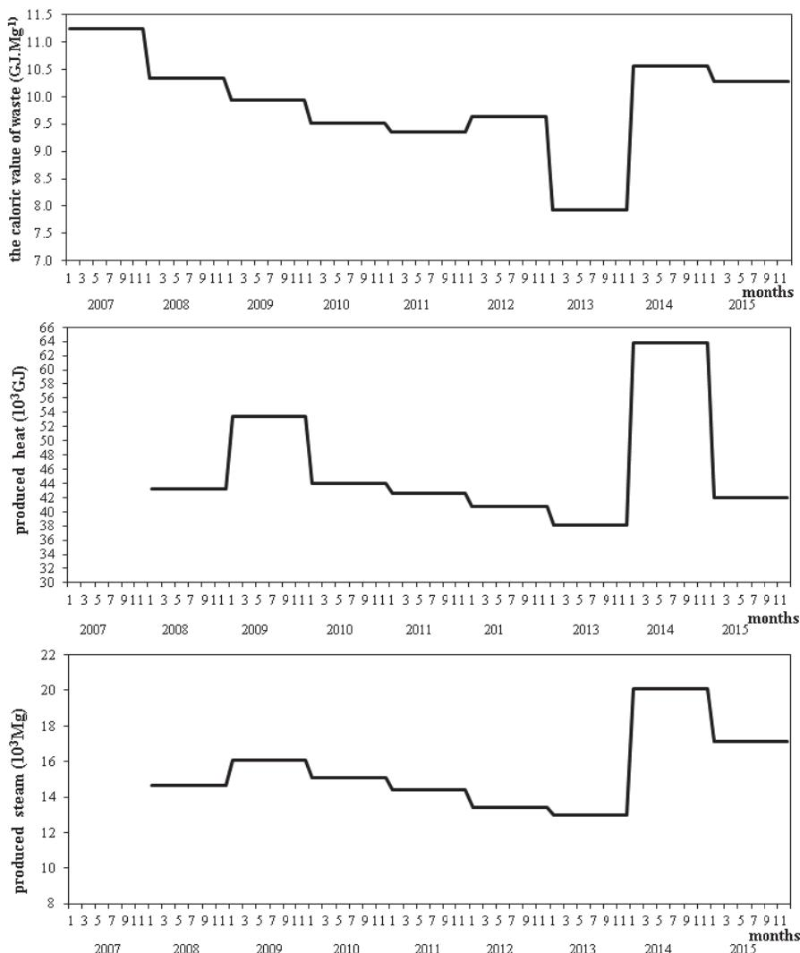
**Fig. 11.** The production of heat and of steam in relation to the net calorific values
