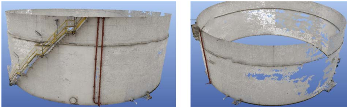
Fig.9. A point cloud acquired from the dense matching (resolution of 4 mm)
