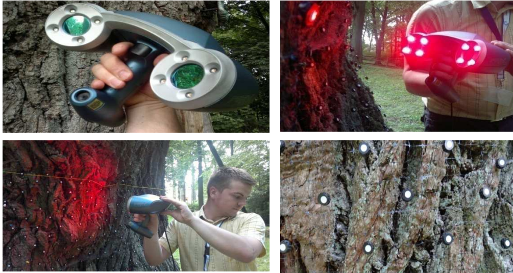
Fig. 4. Precise scanning of the trunk Handy Scan - RevScan (July 2013)
