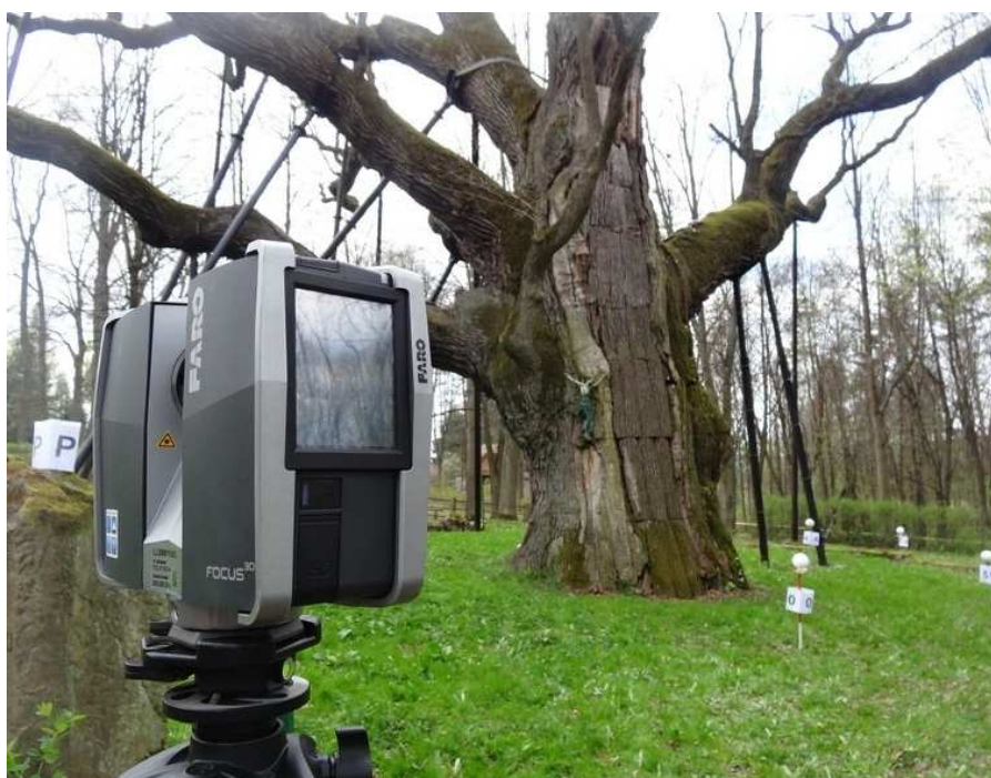
Fig. 2. Selected stand of the FARO FOCUS 3D scanner with the reference spheres
