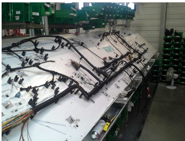
Fig. 4. Assembly table for middle-series and mass production of wire sheaves
