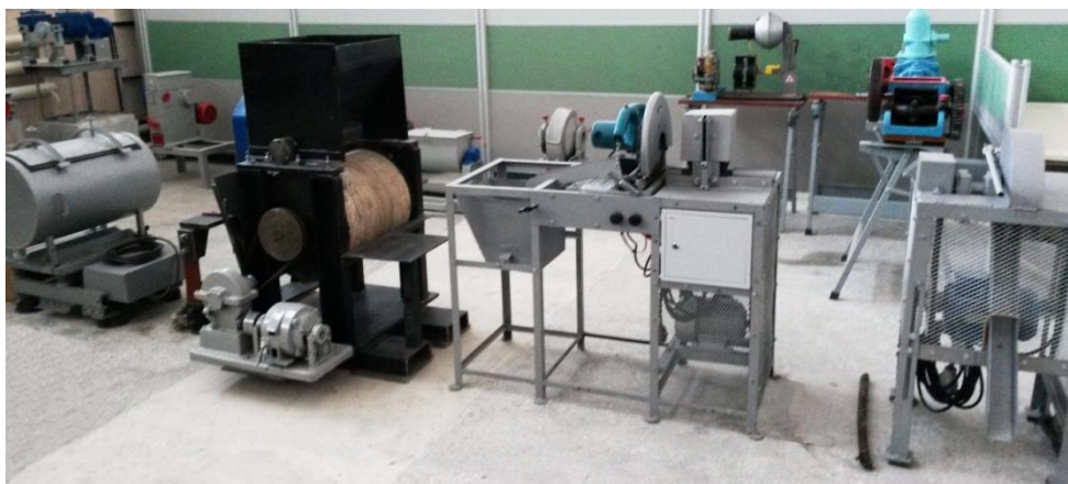
Fig. 6. Experimental samples of the main equipment (in the foreground) of the new production line (from left to right: vibro wash, device for cables separation, semi-automatic for abrasive cables cutting, unit for thermofriction cutting)
