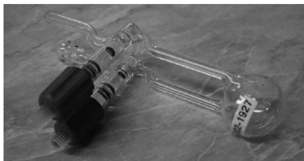
Fig. 2. The glass bubble for the transport of radon activity.
