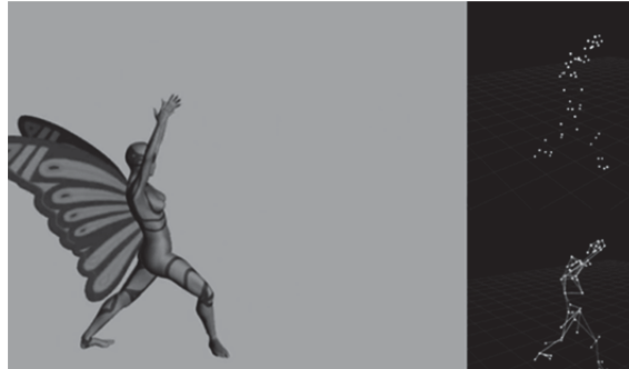
Figure 3. The use of markers to record the movements of points on 3D objects [9]
