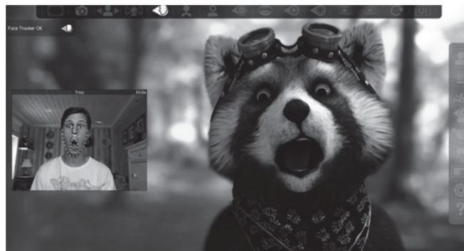
Figure 6. Scanning facial expressions and transposing them on the face of an avatar [10]
