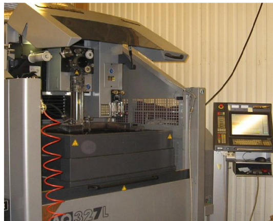
Fig. 2. Front view of the workstation – electrical discharge machine Sodick AQ 327 L
