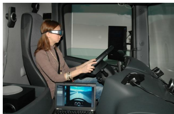
Fig. 6. Research with the use of high-class driving simulator and on-head eye-tracking device
