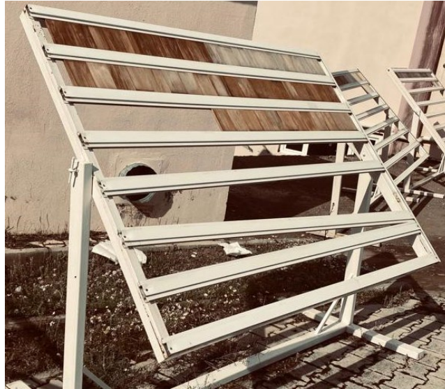
Fig. 1. Weathering test apparatus
