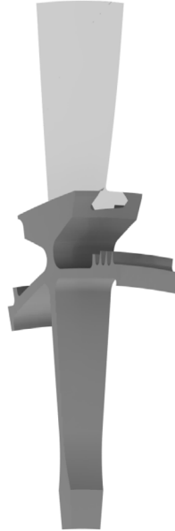
Fig. 6. Cyclic symmetry model of the compressor 3 rd rotor stage
