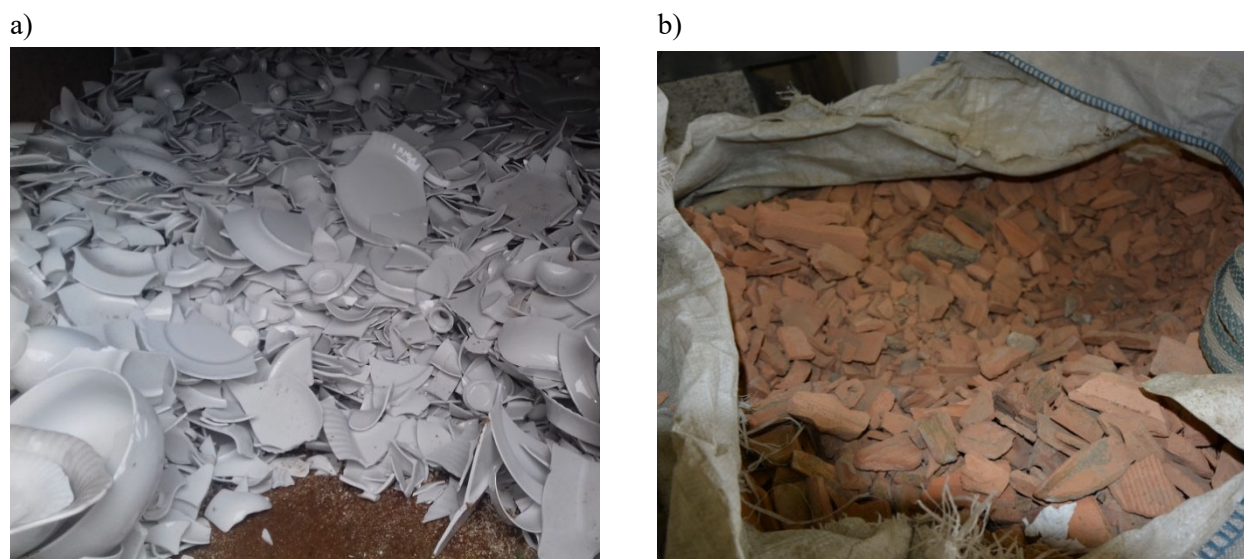
Fig. 1. a) Waste from a) porcelain factory b) pre-crushed waste from ceramic hollow bricks
