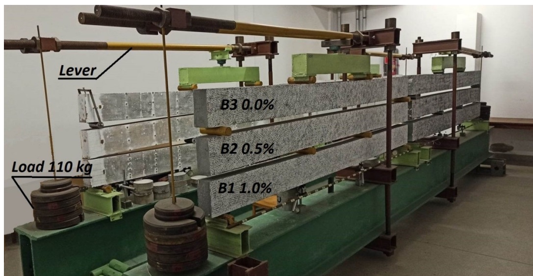
Fig. 4. Stands for testing rheological properties of cement composites based on waste aggregate. Stage I, mixtures RCf, RCc, WCf, WCc
