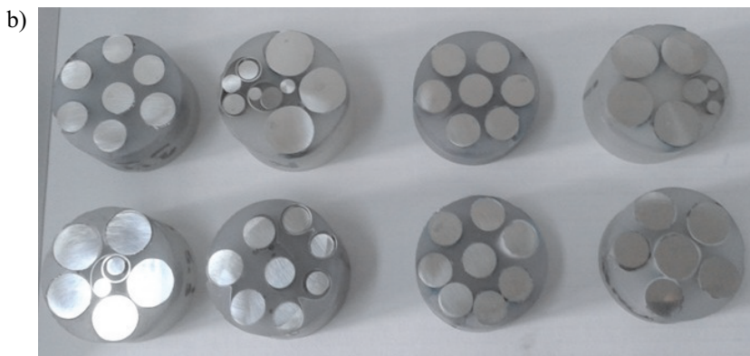
Fig. 4. Struers LaboPol-5 grinding and polishing machine with LaboForce-3 specimen mover (a) and metallographic specimens after final polishing (b)
