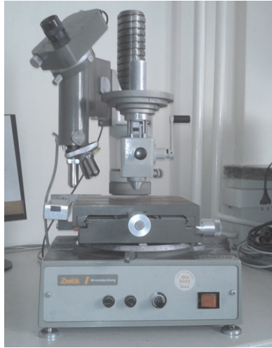
Fig. 5. Zwick 3212002 hardness tester used for HV measurements
