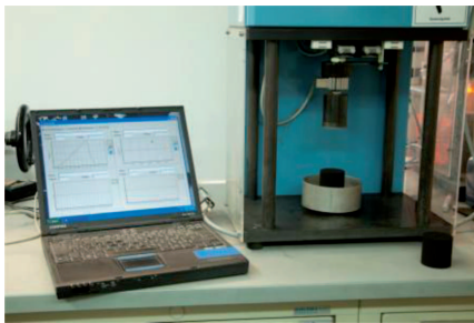
Fig. 11. Deformation equipment of Boenisch
