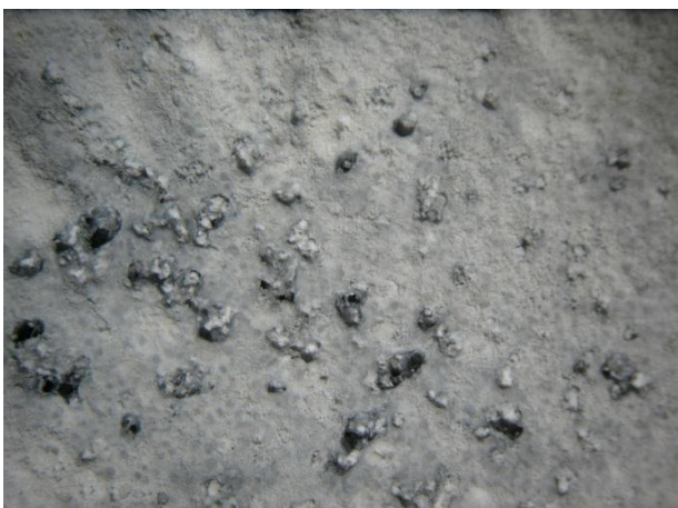
Fig. 8. Surface topography of alloy 3 sample (after 6 h of being immersed in 5% HCl solution, 7x)
