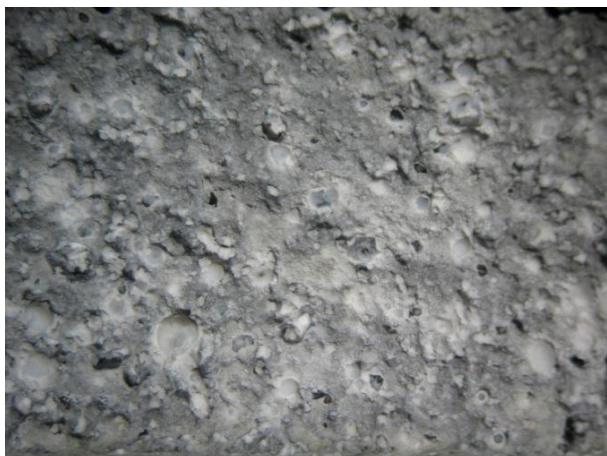
Fig. 7. Surface topography of alloy 2 sample (after 6 h of being immersed in 5% HCl solution, 7x)
