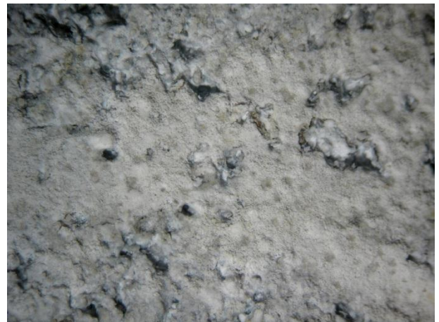
Fig. 6. Surface topography of alloy 1 sample (after 6h of being immersed in 5% HCl solution, 7x)
