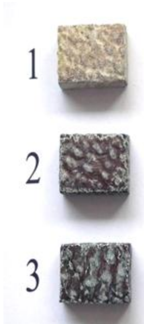
Fig. 3. Corrosion behaviour of Mg-Li alloy samples after 6 h of being immersed in 5% HCl solution
