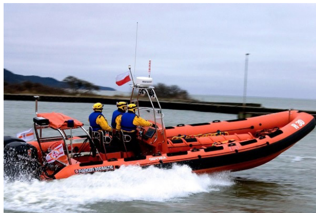
Ryc. 18. Łódź ratownicza RIB typu Baltic Parker 900 [9] Fig. 18. Rescue boat RIB, type Baltic Parker 900 [9]
