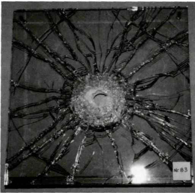
Figure 8. Penetration of 24-mm laminated safety glass by a 0.625-kg projectile according to prEN 12415 (CEN, 1996b), projectile velocity: 35 m/s.
