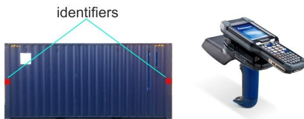
Fig. 6. Identification of location of the places of the parts of the drilling pipe: a) arrangement of identifiers on the container, b) reader of the firm Intermec CK3
