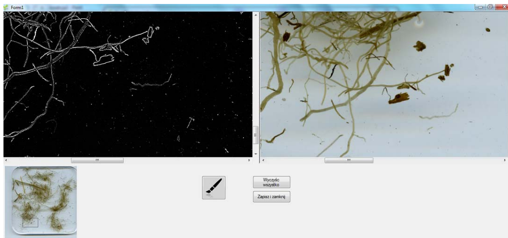
Figure 5. Image correction module with the original image and visible image of the detected edges
