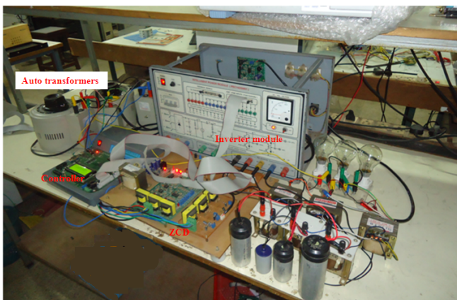
Fig. 3. ZSI-UPQC experimental set-up
