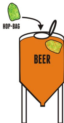
Figure 1. Hop bag addition into fermentation tank. Source: own work based on [11]
