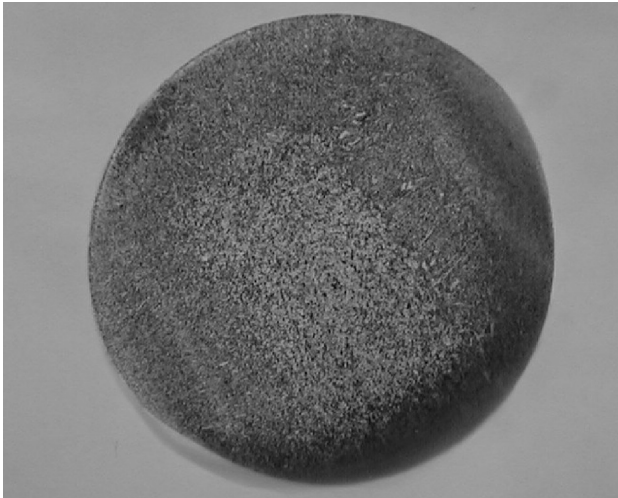
Fig. 6. Presentation of the sulfur segregation on the cross-section of a coupling screw – Baumann print [own work]
