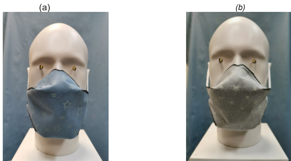
Fig. 2. Models of anti-smog half-masks: (a) – model A – sample 1, the outer layer printed with a phosphorescent open star pattern, (b) – model B – sample 2, the outer layer printed with a phosphorescent solid star pattern
