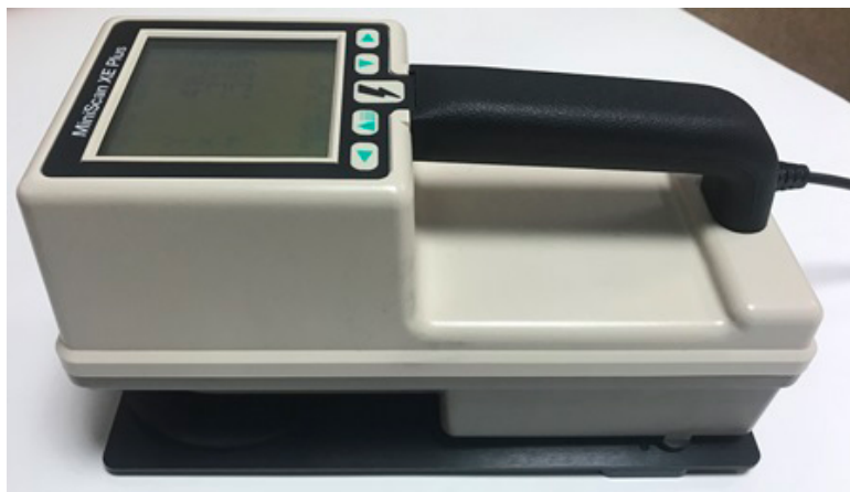
Fig. 4. MiniScan XE Plus reflectometer (USA) used for determining the reflectance coefficient and chromaticity coordinates
