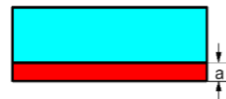
Case II Fig. 2. Extended surface crack: a – length of the crack
