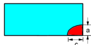
Case V Fig. 5. Quarterelliptical corner crack: a – length of the crack; c – its width
