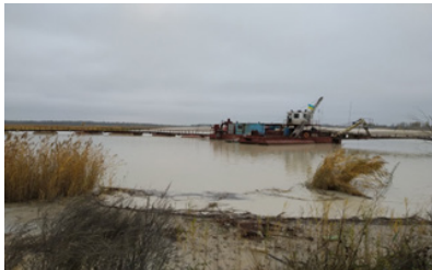
Fig. 7. Development of man-made deposit of titanium-zirconium ores by hydromechanized method
