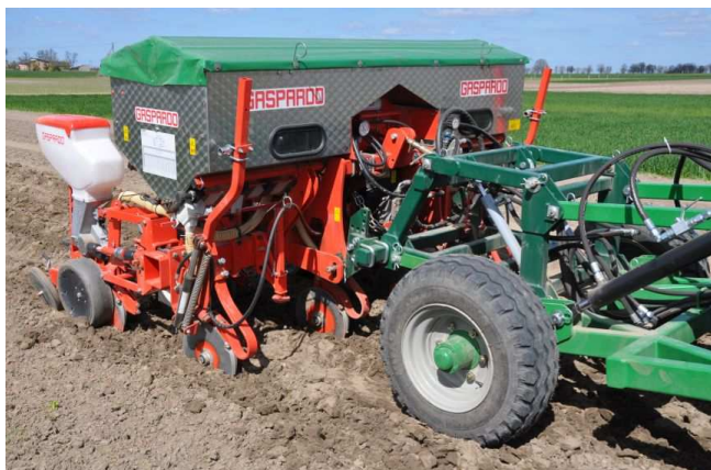
Fig. 2. Corn seeder mounted on unit coupler (second working module of research model)
