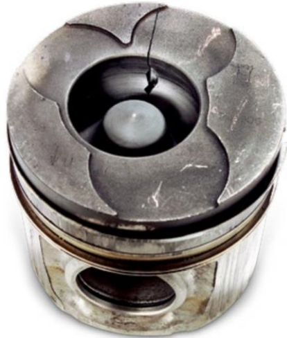
Fig. 4. Diesel engine piston with a crack on the bottom [21]
