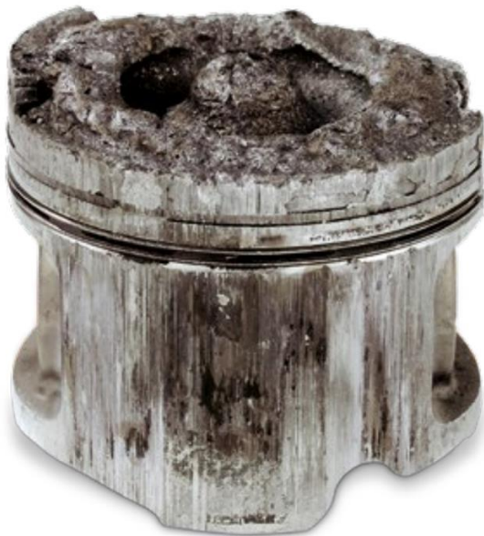
Fig. 5. Diesel engine piston with a melted bottom [21]
