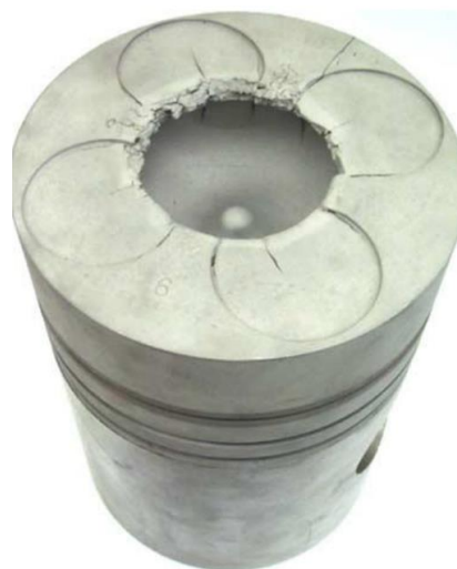
Fig. 3. Diesel engine piston with a chipped edge of the combustion chamber [20]
