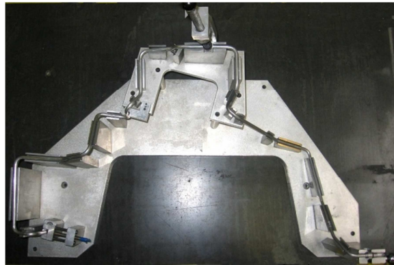
Fig. 3. Verification of bended elements; example check-gauge
