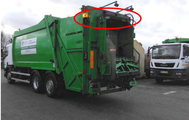
Fig. 7. Equipment emitting variable yellow light - back of the vehicle
