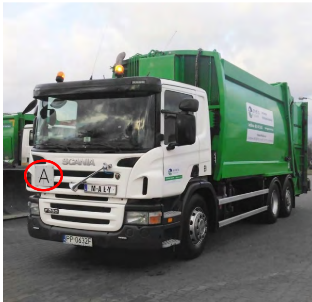
Fig. 5. Panel with letter „A” used for labeling waste vehicles in Germany
