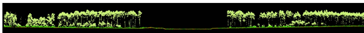
Fig. 4. An example of a cross section made from a point cloud obtained from airborne laser scanning running through the middle of the water reservoir; source: own elaboration
