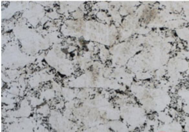
Fig. 9. Sample B. Non-etched and oxides and pores (magnification 100x)
