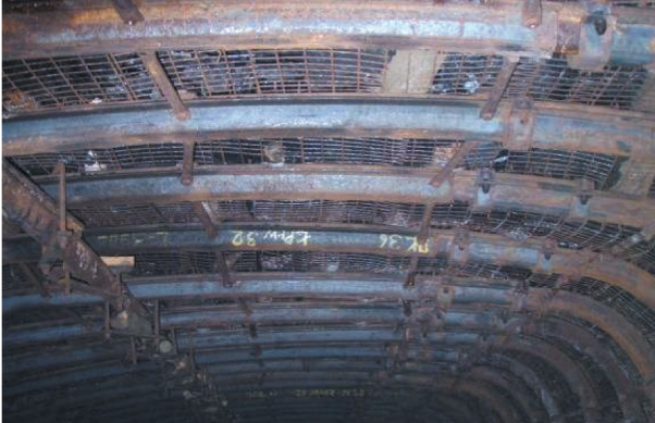
Fig. 47. Development drift secured by means of the ŁPrw support
