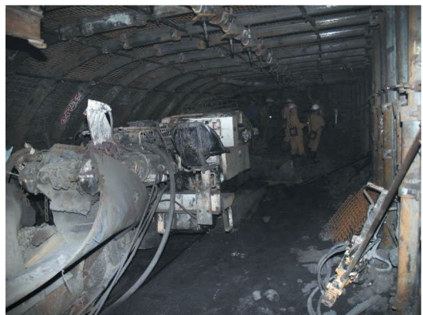
Fig. 20. Longwall closure drift secured by means of the ŁPro/B support
