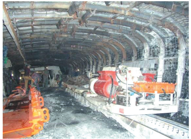
Fig. 42. Longwall equipment in a development drift secured by means of the ŁPrP variant K support
