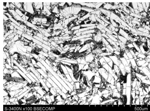
Fig. 3. The structure of bonded magnets based on Nd_{11}Fe_{77}Co_5B_6 powder after biencapsulation with Ni-P/epoxy resin
