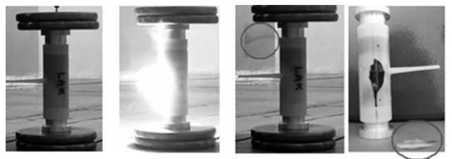
Fig. 3. Surface discharge on the surge arrester and damage of the polyamide housing [6]
