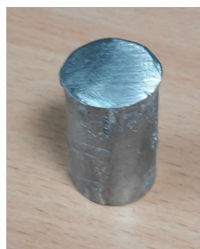
Fig. 3. Composite cast \phi=20\text{mm} , h=30\text{mm} : matrix TBC20, reinforcement sinter alumina powder
