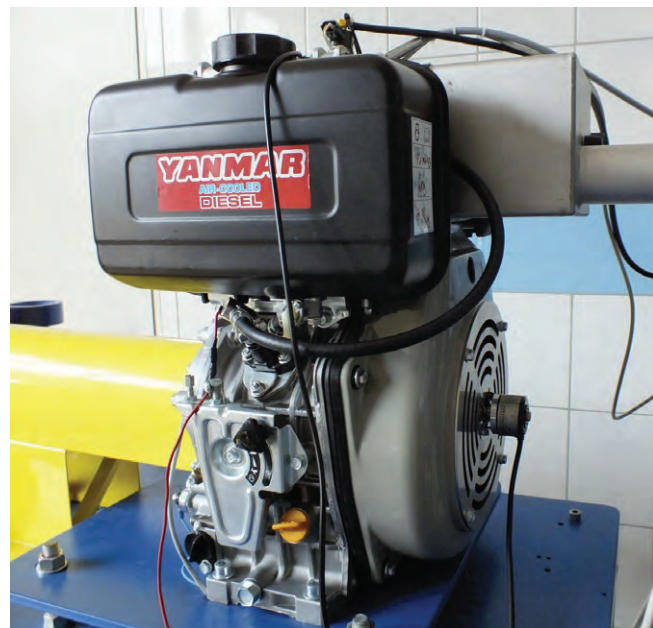
Fig. 4. View of the tested engine with mounted encoder and suction valve position sensor
