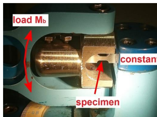
Fig. 3. Method of restrained and specimens loaded
