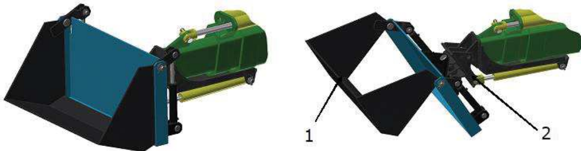
Fig.7. Multi-purpose bucket – general view 1 – bucket, 2 – articulating joint
