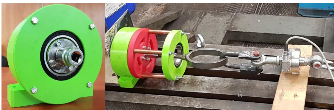
Fig. 4. 3D printout of the magnetic coupling, view of the test stand [10]
