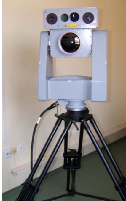
Fig. 2. The turntable together with the sensors
