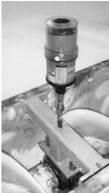
Fig. 7. The appearance of the slide bearing casing in the screw conveyor with the grease dispenser
