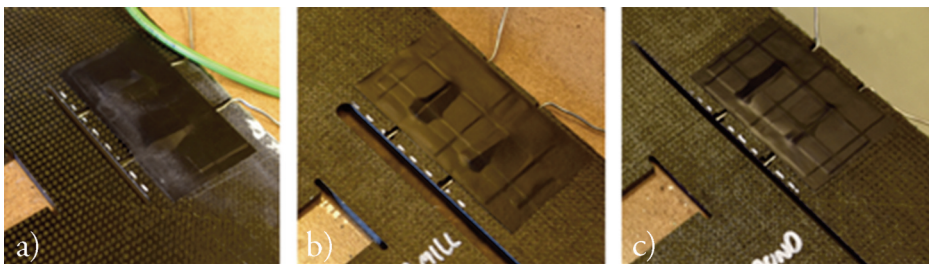
Figure 4. Grooves machined next to thermocouples using three tools: a) Tool 1, b) Tool 2, c) Tool 3 [author's materials]
