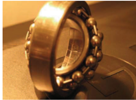
Fig. 13. Evolution of rolling bearing degradation with artificial defect on the outer raceway after its operation under loading of 28 N
