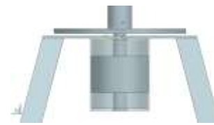
Fig. 3. CAD model of the connection of the generator with the wind turbine rotor and supporting structure
